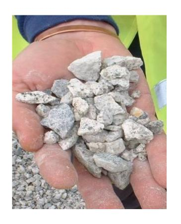
•Local virgin aggregates will have lower eCO<sub>2</sub> than RA transported longer distances (over 15km by road)
